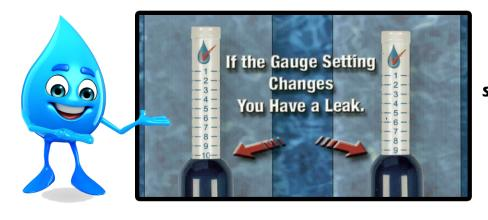
If you lose more than the seepage rate of 1/8" within 24hrs, you have a leak that should be located and repaired.
