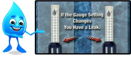
If you lose more than the seepage rate of 1/8" within 24hrs, you have a leak that should be located and repaired.
